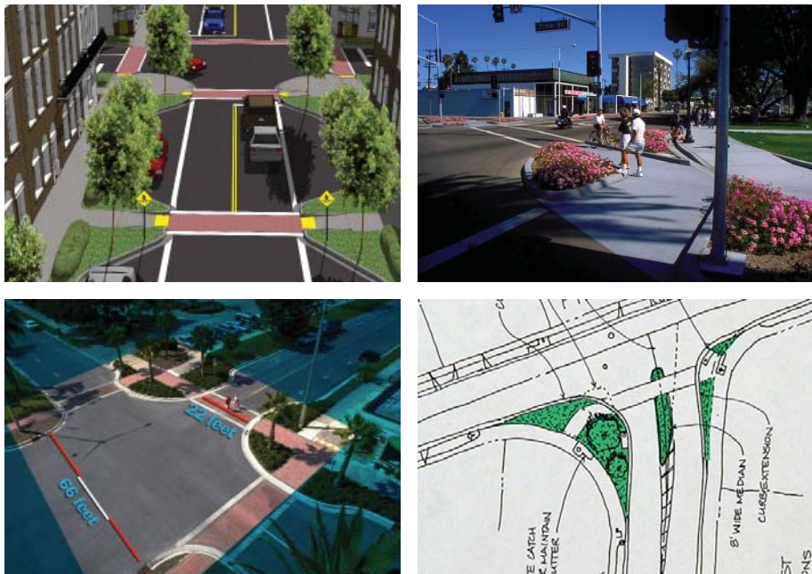
Above: Examples are shown of some ways curb extensions can be applied to reduce crossing distances for pedestrians, improve the geometry of intersections and keep vehicle speeds low—and safe—through turns.
