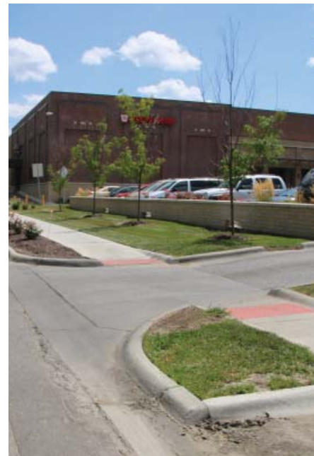
Above left: A grocery store driveway is narrow, which helps slow cars down and keeps crossing distances short for pedestrians. Top right: where sidewalks and driveways intersect, the design should favor the pedestrian.
